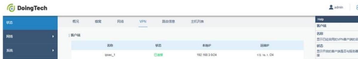
This screenshot is identical to the one above, showing the DoingTech interface with the 'Network' tab selected. The 'Help' panel is also visible, and the '客户端' table shows the same connection information for 'ipsec\_1': 已连接 (Connected), 192.168.3.0/24, 172.16.1. /24.
